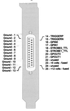
Figure 4.2 The I/O connector
